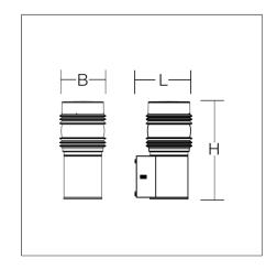
Attractive wall luminaire with innovative housing design and high-quality LED optics. Housing made of corrosion-resistant die-cast aluminium, seawater resistant powder-coated. With membrane valve as a standard to avoid condensed water. Mouth-blown luminaire glass, clear, drum lens shape. Fixing on the wall outside the sealed volume, drill hole deviations can be compensated. Screwless luminaire fixing via RZB Gravolock® System.
