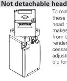
To make head adjustment safer and smoother, these switches are equipped with a special head to body coupling system. This system makes it impossible to remove the head from the device even during adjustment, thus rendering the use of one-way screws unnecessary for locking the head in position once adjustment is complete. This solution is available for the FR, FX and FK series.
