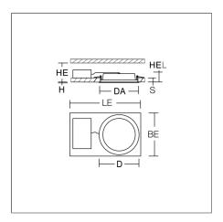
Flexible round recessed multifunction downlight. Luminaire for escape route illumination. Housing: sheet steel, powder-coated. Luminaire frame: aluminium, powder-coated. Diffuser made of non-yellowing plastic (PMMA), opal. LED backlight technology for homogeneous illumination of the entire light-emitting surface. Ceiling installation with spring system. Including separate LED converter with connecting cable 250 mm.
