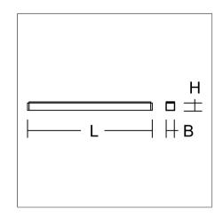
Ceiling luminaire with slim design. Housing: extruded aluminium profile, powder-coated. End cap aluminium powder-coated. Diffuser made of non-yellowing plastic (PMMA) microprismatic. Suitable for Ceiling mounting, Wall (surface). External driver with connecting cable.
