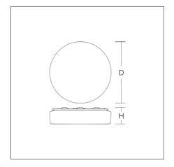
Decorative round surface-mounted luminaire. For escape route illumination. Base: metal, powder-coated. Diffuser made of plastic (polycarbonate), opal, shockproof. Diffuser fastening: patented push system. Suitable for Ceiling mounting, Wall (surface). Driver integrated. Suitable for connection to central battery systems. With AC Control monitoring module for LUXIFAIR central battery units.
