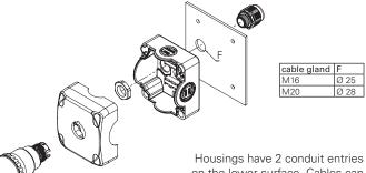
on the lower surface. Cables can be connected via this surface, hiding them from view.
