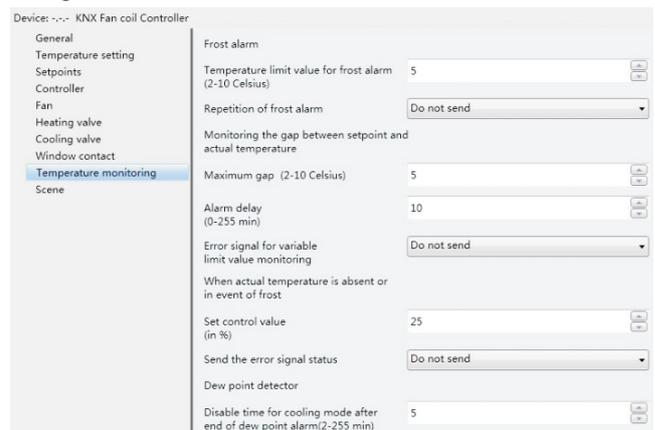
Fig.6.11 Parameter setting window of “Temperature monitoring”
