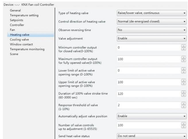
Fig. 6.9 “Heating valve” Parameter setting interface
