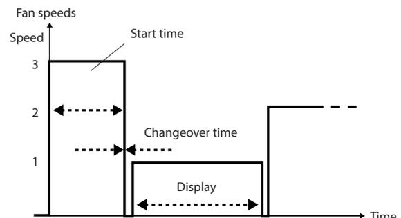
Fig. 6.8 Fan gear shifting mode
