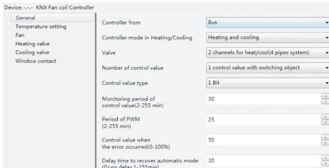
Fig. 6.13 External Control "General" parameter setting interface
