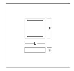
Flexible square surface-mounted multifunction downlight. Luminaire for escape route illumination. Housing: die-cast aluminium, powder-coated. Diffuser made of non-yellowing plastic (PMMA) microprismatic. Suitable for Ceiling mounting, Wall (surface). Self-contained system with automatic self-test and feedback to the RZB monitoring system MULTIDIGIT.
