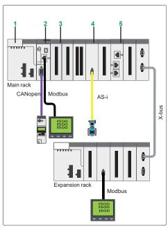
Integrated fieldbus architecture: devices distributed over fieldbuses
