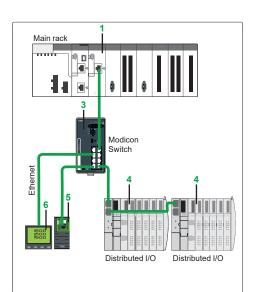
Distributed I/O architecture: devices distributed over Ethernet with BMXNOE0110 module and Modicon Switch
