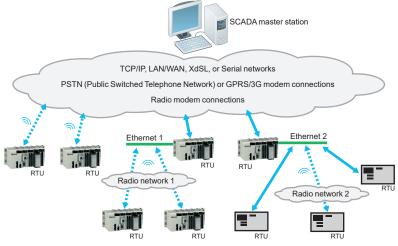
Example of an RTU system architecture
