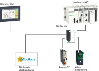
The Modbus serial link is used for master/slave architectures (it is necessary, however, to check that the Modbus services used by the application have been implemented on all relevant devices).
