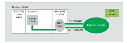
The time synchronization service is based on NTP (*Network Time Protocol*) which is used to synchronize the time of a client or a server on Ethernet from a server or another reference time source (radio, satellite, etc).
