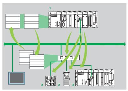
The I/O Scanning Service is used to manage the exchange of remote I/O states on the Ethernet network after a simple configuration operation, with no need for special programming:
