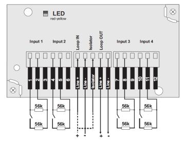
**ATTENTION:** When you use the integrated short circuit isolation module connect one of the "**+Loop**" leads to the "**Isolator**" terminal instead of the "**Line+**" terminal.
