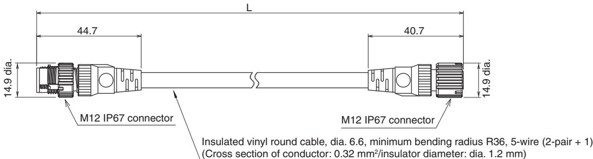
Extended Plug-Socket Cable for Receiver: Cable for extension (F39-JG□B-D, sold separately)
