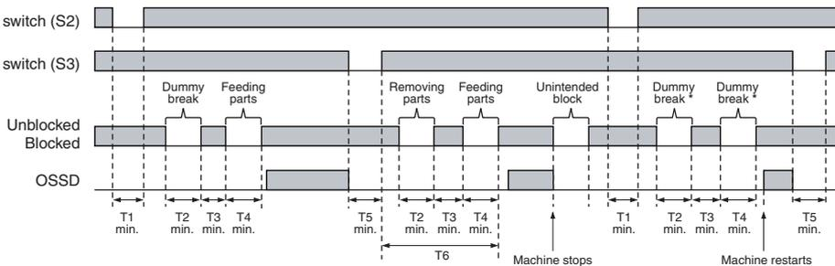
T1: Minimum pressing time of reset switch. Configurable from 100 to 500 ms in 100-ms increments by SD Manager 3.
