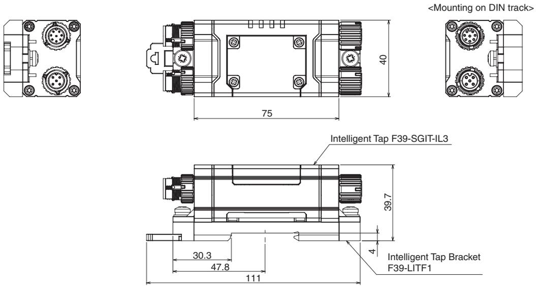
Material: PBT resin (Body parts)
