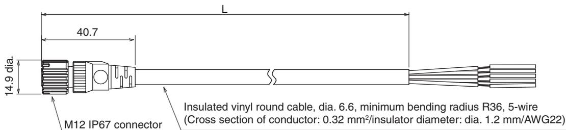
Extended Socket-Straight Cable for Receiver (F39-JG□A-D, sold separately)
