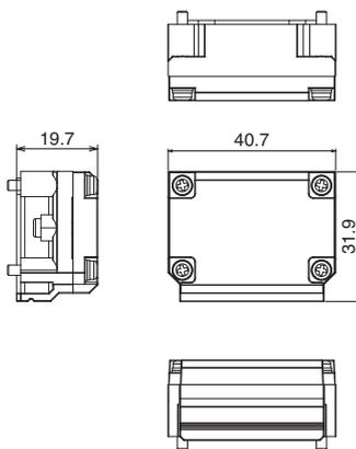
Material: PBT resin (Body parts)
