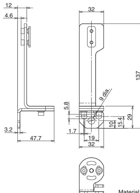
Material: High rolled steel (SPHC)
