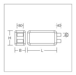
Rectangular wall extension luminaire in classic design. For escape route identification. Housing: aluminium, with plastic corner connectors. Display panels: plastic, opal, with motifs on one side/on both sides. Wall extension Electronic ballast included. Self-contained system with automatic self-test and feedback to the RZB monitoring system MULTIDIGIT. Please indicate legend number when placing your order!
