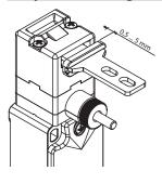
The actuation head of this switch features a wide range of travel. In this way the guard can oscillate along the direction of insertion (4.5 mm) without causing unwanted machine shutdowns. This wide range of travel is available in all actuators in order to ensure maximum device reliability.
