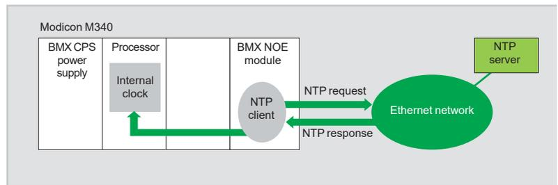
The time synchronization service is based on NTP (*Network Time Protocol*) which is used to synchronize the time of a client or a server on Ethernet from a server or another reference time source (radio, satellite, etc).
