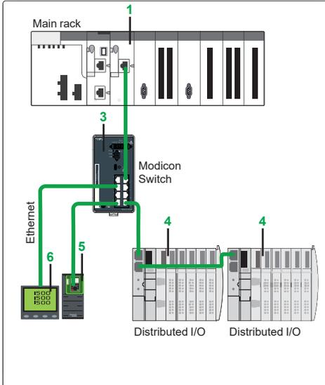
**4** Distributed I/O architecture: devices distributed over Ethernet with BMXNOE0110 module and Modicon Switch
