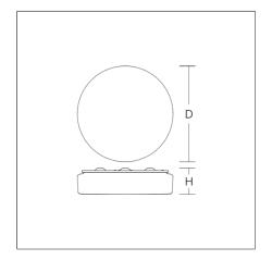
Decorative round surface-mounted luminaire. For escape route illumination. Base: metal, powder-coated. Diffuser made of non-yellowing plastic (PMMA), opal. Diffuser fastening: patented push system. Suitable for Ceiling mounting, Wall (surface). Driver integrated. Suitable for connection to central battery systems. With AC Control monitoring module for LUXIFAIR central battery units.
