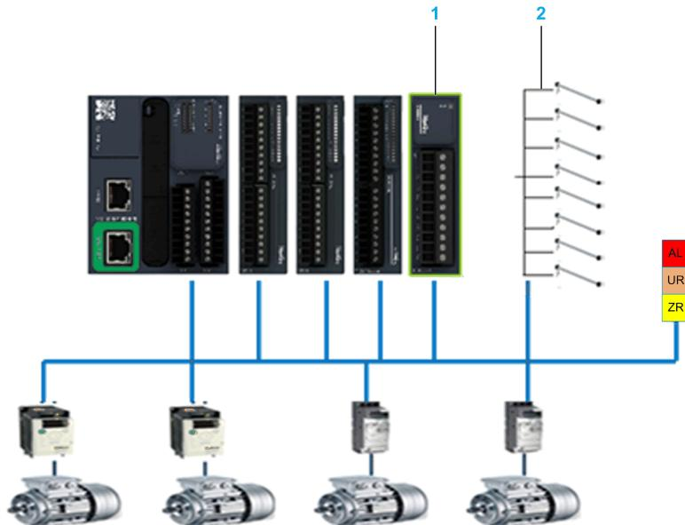
1. Analog output for up to four Variable Speed Drive (VSD)
