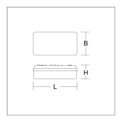
Luminaire for escape route identification. Base: plastic Diffuser: plastic, opal 4 plastic foils with escape route motifs included (ISO 7010). Suitable for Wall (surface). Electronic ballast included. Self-contained system with automatic self-test and feedback to the RZB monitoring system MULTIDIGIT.
