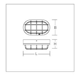
Decorative surface-mounted luminaire for outdoor use. Housing made of corrosion-resistant die-cast aluminium, seawater resistant powder-coated. With membrane valve to avoid condensation. Crystal glass: matt inside. Shadow-free, homogeneous and soft illumination. Base fixing slots outside of gasketed area, drill hole deviations can be compensated. Separate connection compartment for direct connection of rigid cables up to 3 x 2.5 mm². Replaceable LED module.
