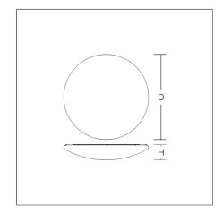
Decorative round surface-mounted luminaire. For escape route illumination. Base: metal, powder-coated. Diffuser made of plastic (polycarbonate), opal, shockproof. Diffuser fastening: patented push system. Suitable for Ceiling mounting, Wall (surface). Self-contained system with automatic self-test and feedback via DALI bus, only to RZB DALI monitoring system.
