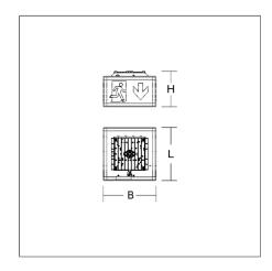
Luminaire for escape route identification. Base: plastic. Frame profile: aluminium anodised. Display panels: plastic, opal, with motifs on three sides. Light emission: downwards. Easy installation by folding mechanism. Electronic ballast included. Self-contained system with automatic self-test and feedback to the RZB monitoring system MULTIDIGIT.
