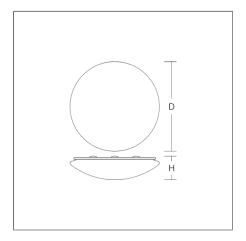
Decorative round surface-mounted luminaire. For escape route illumination. Base: metal, powder-coated. Diffuser made of plastic (polycarbonate), opal, shockproof. Diffuser fastening: patented push system. Suitable for Ceiling mounting, Wall (surface). Driver integrated. Suitable for connection to central battery systems. With AC Control monitoring module for LUXIFAIR central battery units.
