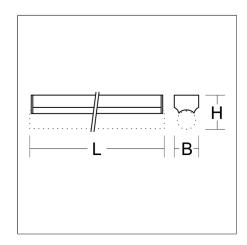
ISO striplight for linear lamps. Base: plastic. Lamp contacts disconnection during lamp replacement. Light source must be ordered separately.
