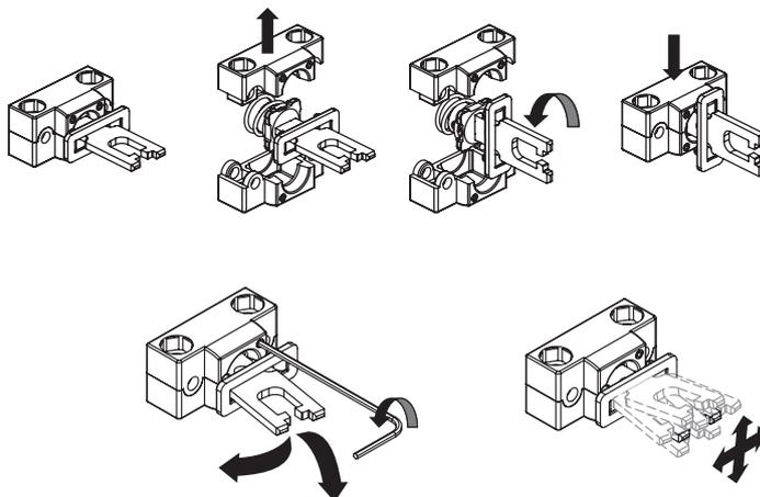
Jointed actuator for guards with poor alignment, adjustable in two dimensions for small doors; can be mounted in various positions. The metal fixing body has two pairs of bore holes; it is provided for rotating the working plane of the actuator by 90°.
