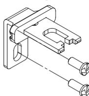
As required by ISO 14119, the actuator must be fixed immovably to the guard frame. Pan head safety screws with one-way fitting are available for this purpose. With this screw type, the actuators cannot be removed or tampered by using common tools. See accessories on page 419.
