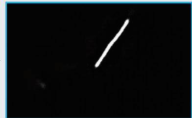
Detection image Can detect a scratch only
