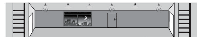
4 After stand-by period, the lamps will be switched off if no movement is detected in the detection zone.
