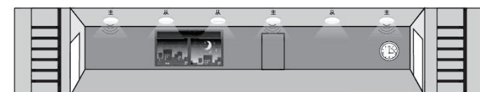
3 If no motion is detected in the detection zone, all lamps will be synchronously dimmed to a low light level after hold time.
