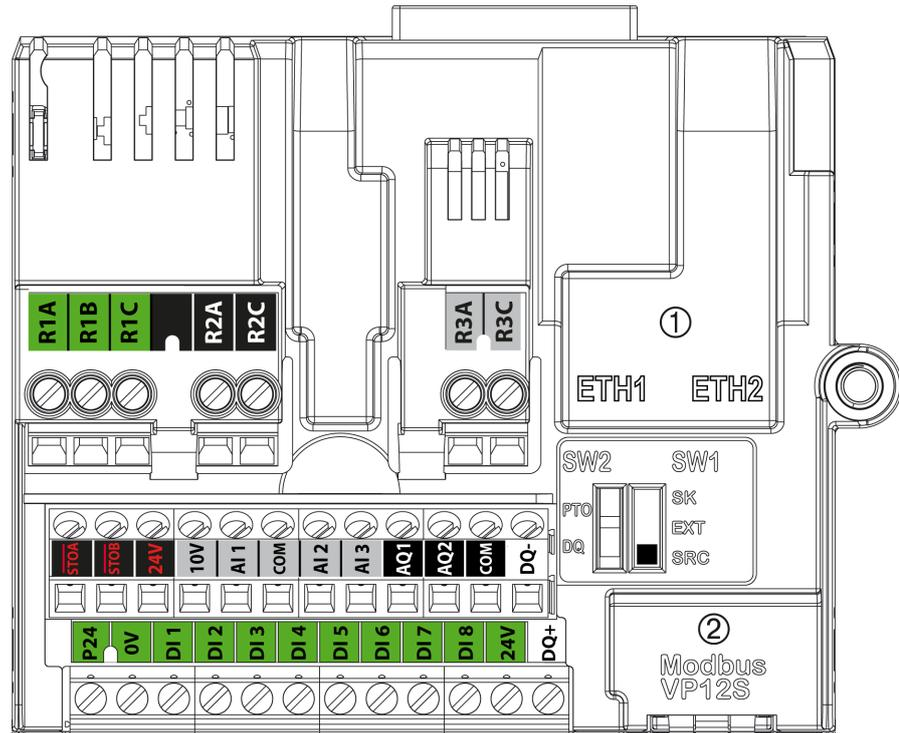
① Ethernet Modbus TCP, ② Serial Modbus
