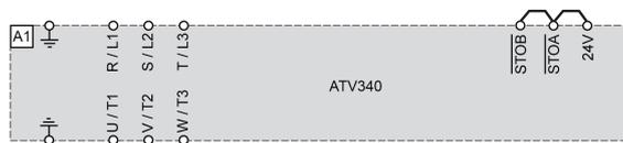
When not used for functional safety the STO inputs should be connected to 24V.
