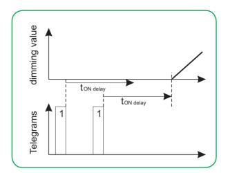
Value: not retriggerable If the channel receives an ON telegram, the ON delay will be started. If a new ON telegram then follows while the delay time is running, this will be ignored and the ON procedure will be executed after the delay time that was initially started has expired. However, the value of the new telegram is saved as the new setpoint, which will be activated after the delay period has expired.
