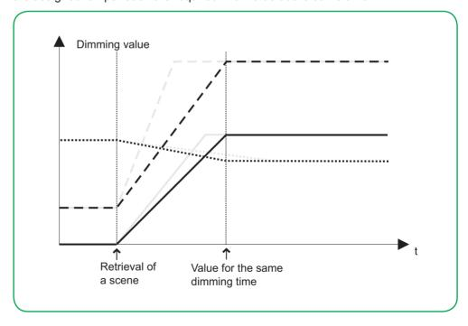
You enable the function globally for the device via a parameter, set an appropriate dimming time after enabling and then activate the *Same dimming time* function for each dimming channel.
