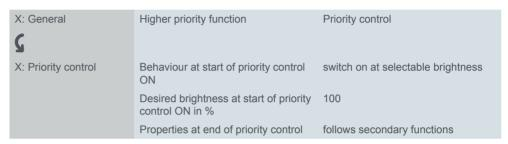
After priority control is activated, the dimming time reduction settings for higher priority functions are used to dim to 100%.
