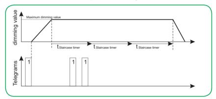
You can limit the possible running time using the *Max. number of time accumulations* parameter.
