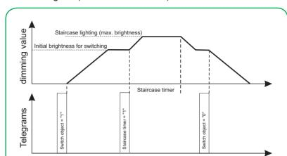
The brightness of the logic operation result and the dimming speed are defined by the last telegram (see the charts below).
