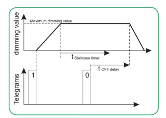
If you have selected the parameter value without manual OFF, the staircase lighting function will not be interrupted when a telegram with the value "0" is received, but will continue to run normally until the staircase lighting time has expired.
