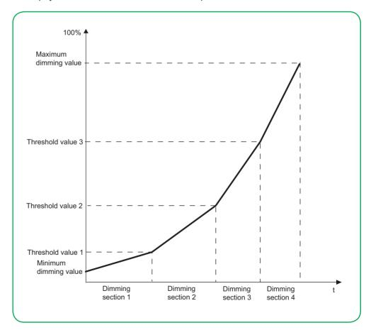
The base dimming curve is divided into **four dimming sections**. You can set individual times for each dimming section. The sum of these times is the total time for a dimming process.
