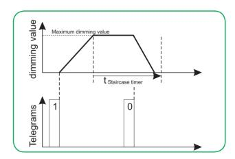
If an OFF delay has also been parameterised, this delay will now be active, and the output will only switch off after the delay time has expired.
