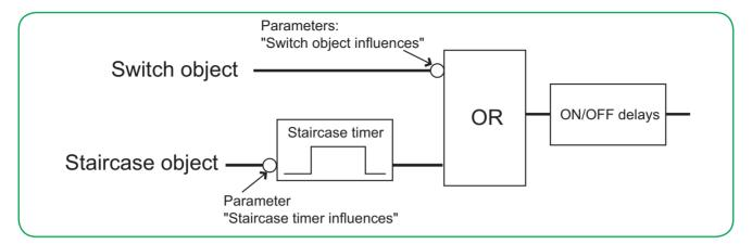
You can invert the effect of the two object values on this logic operation using parameters.
