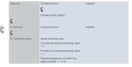
First, select how you want the output to react when a new object value is received for the central object. If you wish to set a variable brightness, you can specify the required values other parameters.
