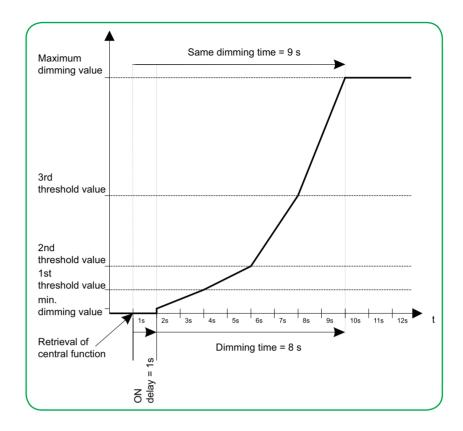
The dimming curve is compressed so that the total time corresponds to the value of the set Same dimming time: New dimming time = Same dimming time minus delay time.
