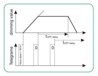
Switch-OFF telegram during dimming process
