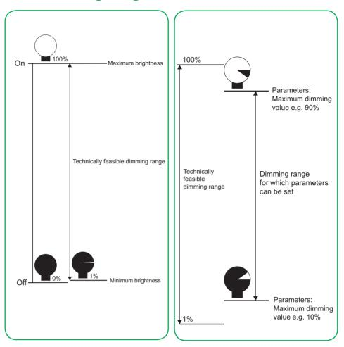
The technical dimming range is defined by the range between the minimum and maximum brightness of a lamp, and can be set with the aid of a dimmer.
