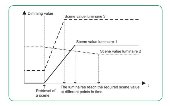
Same dimming time can be used to synchronise the different dimming times of the channels so that all the channels reach their setpoint values at the same time.
