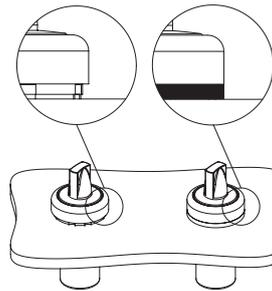
The shaped ring can be used when no label holder or other devices are applied; it prevents dirt and other residues from settling between the potentiometer and the panel or housing.
