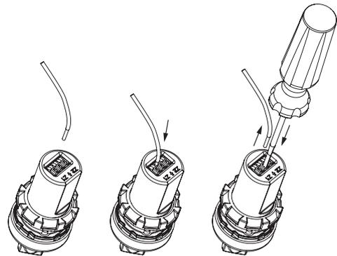
The potentiometer is provided with a three-pole terminal board with PUSH-IN type spring-operated connection. This technology allows a very handy quick wiring procedure. The wire is simply inserted into the appropriate hole, without the need for any auxiliary tooling, through the use of rigid or flexible wires with crimped wire-end sleeve. Release is obtained by pressing the appropriate wire-releasing button.
