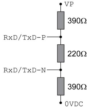
If the device is at the end of the network, use a Profibus connector with terminating resistor.
