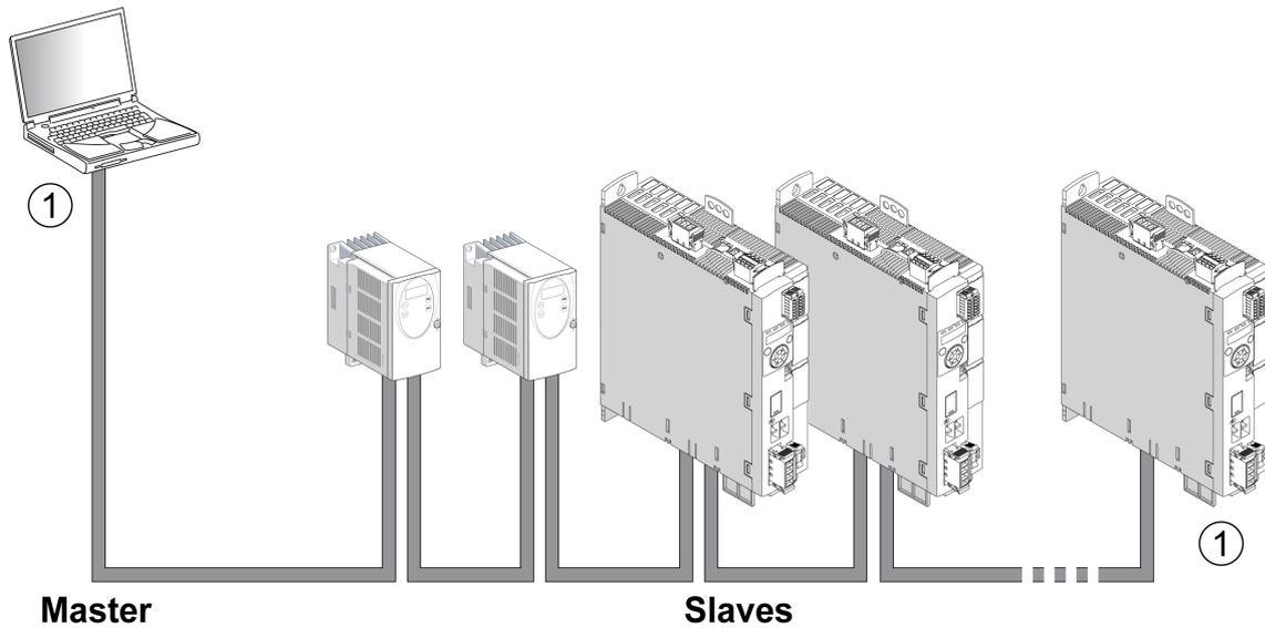
1 Both ends of the fieldbus must be terminated with a terminating resistor.
