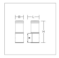
Attractive wall luminaire with innovative housing design and high-quality LED optics. Housing made of corrosion-resistant die-cast aluminium, seawater resistant powder-coated. With membrane valve as a standard to avoid condensed water. Luminaire head made of die cast aluminium, powder-coated, with opal cylinder (glass). Fixing on the wall outside the sealed volume, drill hole deviations can be compensated. Screwless luminaire fixing via RZB Gravolock® System.
