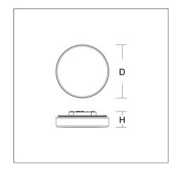
Decorative round surface-mounted luminaire. For escape route illumination. Base: metal, powder-coated. Diffuser made of non-yellowing plastic (PMMA), opal. Diffuser fastening: patented push system. Suitable for Ceiling mounting, Wall (surface). Self-contained system with automatic self-test and feedback to the RZB monitoring system MULTIDIGIT.
