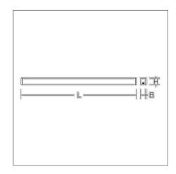
Linear ceiling and wall luminaire for aesthetically sophisticated lighting. Housing: extruded aluminium profile, powder-coated. End cap aluminium powder-coated. Diffuser made of non-yellowing plastic (PMMA), opal. Suitable for Ceiling mounting. LED unit with integrated converter interchangeable and removable. Suitable for through-wiring. With sensors or as a safety luminaire on request.
