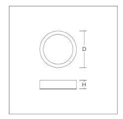
Flexible round surface-mounted multifunction downlight. Luminaire for escape route illumination. Housing: die-cast aluminium, powder-coated. Light guide and diffuser made of non-yellowing PMMA, opal matt. Suitable for Ceiling mounting, Wall (surface). Self-contained system with automatic self-test and feedback via DALI bus, only to RZB DALI monitoring system.
