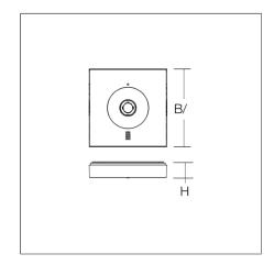
Flat, square surface-mounted luminaire. For escape route illumination. Housing: plastic (polycarbonate). Cover: polycarbonate. Plastic lenses for area lighting and escape route illumination included in scope of delivery. Lenses can be replaced without tools. Suitable for connection to central battery systems.
