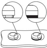
The shaped ring can be used when no label holder or other devices are applied; it prevents dirt and other residues from settling between the indicator and the panel or housing. This turns out to be particularly useful in the sectors where high standards of cleanness and hygiene are required.
