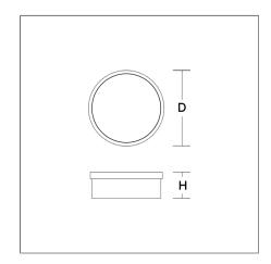
Round surface-mounted luminaire in classic design. Base: plastic. Diffuser: plastic (polypropylene), opal, satin finish. Diffuser fastening: spring system. Suitable for Ceiling mounting, Wall (surface). IP 43 ceiling mounting, IP 44 wall mounting.
