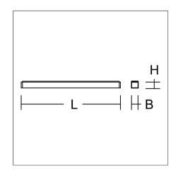
Ceiling and wall luminaire with slim design. Housing: extruded aluminium profile, powder-coated. End cap aluminium powder-coated. Diffuser made of non-yellowing plastic (PMMA), opal. Suitable for Ceiling mounting, Wall (surface). External driver with connecting cable.
