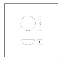
Decorative round surface-mounted luminaire for indoor and outdoor use. Base: plastic. Diffuser made of plastic (polycarbonate), opal, shock-proof. Diffuser fastening: spring system. Suitable for Ceiling mounting, Wall (surface). Slave luminaire. Can only be operated in combination with corresponding master luminaire. IP 43 ceiling mounting, IP 44 wall mounting.
