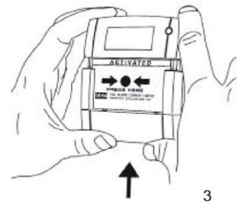
**TO REPLACE GLASS/RESETTABLE ELEMENT**
