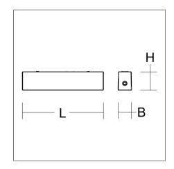
Rectangular surface-mounted luminaire in classic design. For escape route illumination. Housing: shockproof plastic (polycarbonate). Lens, plastic, for ideal light distribution on escape route. Suitable for Ceiling mounting, Suspension cable/chain, Wall (surface). Large cable entry space. Suitable for through-wiring. Driver integrated. Suitable for connection to central battery systems. With AC Control monitoring module for LUXIFAIR central battery units. Suspension set as accessory.
