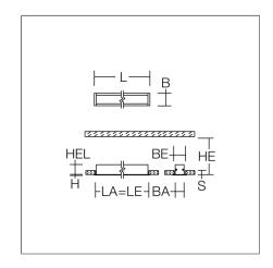
Linear recessed ceiling and wall luminaire for aesthetically sophisticated lighting. Housing: extruded aluminium profile, powder-coated. End cap aluminium powder-coated. Diffuser made of non-yellowing plastic (PMMA), opal. Ceiling installation with pre-assembled SBS mounting system. Suitable for Recessed ceiling mounting, wall (recessed). LED unit with integrated converter interchangeable and removable. With sensors or as a safety luminaire on request.
