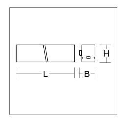
Linear wall luminaires. Housing: extruded aluminium profile, powder-coated. End cap aluminium powder-coated. Diffuser made of non-yellowing plastic (PMMA), opal. Direct light emission. Suitable for Wall (surface). LED unit with integrated converter interchangeable and removable. Suitable for through-wiring. With sensors or as a safety luminaire on request.
