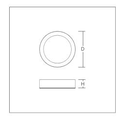
Ultra thin surface mounted downlight. Cylinder housing sheet steel, powder-coated. Bezel ring: die-cast aluminium, powder-coated. Light-guide and diffuser made of non-yellowing PMMA, prismatic. Suitable for Ceiling mounting, Wall (surface). Driver integrated.
