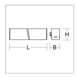
Linear wall luminaires. Housing: extruded aluminium profile, powder-coated. End cap aluminium powder-coated. Diffuser made of non-yellowing plastic (PMMA), opal. Direct 50%, indirect 50% light emission. Suitable for Wall (surface). LED unit with integrated converter interchangeable and removable. Suitable for through-wiring. With sensors or as a safety luminaire on request.
