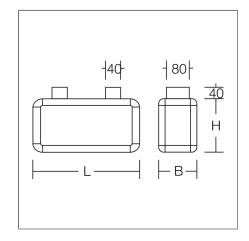
Rectangular surface-mounted luminaire in classic design. For escape route identification. Housing: aluminium, with plastic corner connectors. Display panels: plastic, opal, with motifs on one side/on both sides. Driver integrated. Suitable for connection to central battery systems. Please indicate legend number when placing your order!
