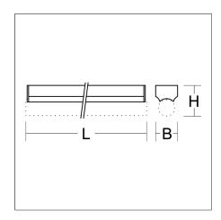
Aluminium striplight for linear lamps. Base: extruded anodised aluminium profile. End caps: plastic. With push button switch. Lamp contacts disconnection during lamp replacement. Light source must be ordered separately.
