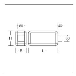
Rectangular wall extension luminaire in classic design. For escape route identification. Housing: aluminium, with plastic corner connectors. Display panels: plastic, opal, with motifs on one side/on both sides. Wall extension Driver integrated. Suitable for connection to central battery systems. With AC Control monitoring module for LUXIFAIR central battery units. Please indicate legend number when placing your order!
