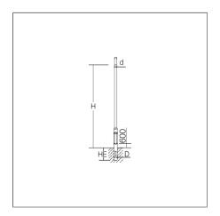
Cylindrical stepped pole made of steel according to DIN EN 40. Hot-dip galvanised in compliance with DIN EN ISO 1461. Wall thickness 3 mm. Flush pole door, 85 x 400 mm. Triangular lock, other locks on request. C-slot with two sliding nuts M6 and earthing thread M8. Cable hole 50 x 150 mm (UKK 500 mm below level).
