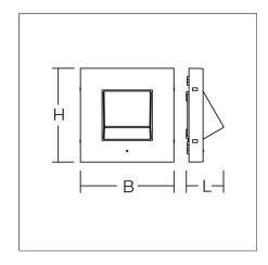
Wall luminaire for escape route illumination. Base: die-cast aluminium, powder-coated Cover: polycarbonate. With plastic lenses for area lighting. Vertical swivel. Driver integrated. Suitable for connection to central battery systems. With AC Control monitoring module for LUXI-FAIR central battery units. Luminaires with limited surface temperature in accordance with EN 60598-2-24 for use in environments in which a deposit of conductive dust on the luminaire can be expected.
