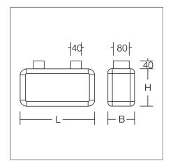
Rectangular surface-mounted luminaire in classic design. For escape route identification. Housing: aluminium, with plastic corner connectors. Display panels: plastic, opal, with motifs on one side/on both sides. Electronic ballast included. Self-contained system with automatic self-test. Please indicate legend number when placing your order!
